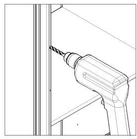
**Step2.**Using the marked locations, drill pilot holes through the profile into the end panels.
