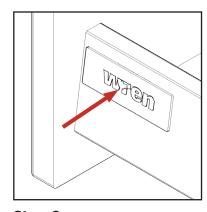
**Step 3**Press the cover cap against the drawer side to secure it in place. Repeat on the opposite side.
