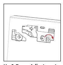
**Up & Down Adjustment**Turn screw shown to **adjust**drawer frontal **up & down.**
